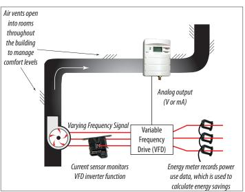
Using a VFD in HVAC monitoring allows smart control of the entire system. The peripheral devices offer a total picture of the system status and the power usage profile. Optimum conditions are maintained, while equipment operation costs are kept to a minimum, ensuring long-term cost savings.
